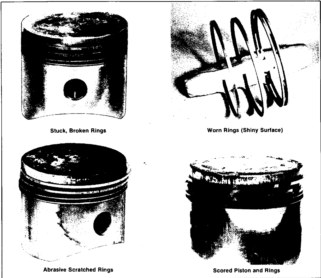
Figure 7-8. Some Common Forces of Piston and Ring Damage
