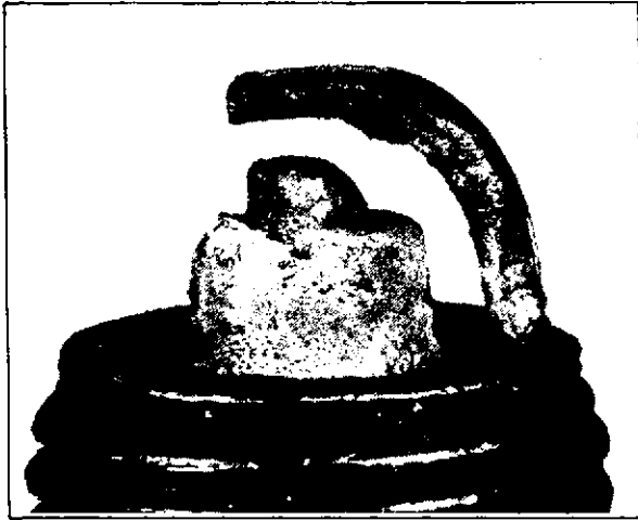
Worn Out: On a plug which has been in service too long, the center electrode will be rounded off and the gap will be eroded .010" or more than the original setting. Replace worn plugs as they will require excessive voltage to fire properly.
